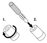
Connect the amplifier to each speaker as shown in the illustration below.
